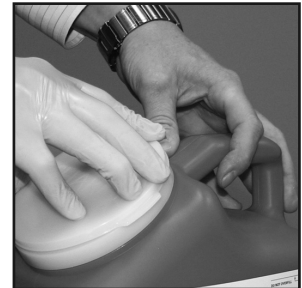
Fig. 4: Close lid by snapping firmly over opening. Make sure lid is tightly sealed prior to packaging.
