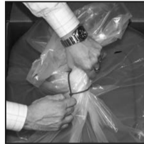
Fig. 7: Pull second bag up around the 20-g or 30-g and close with tiewrap.
